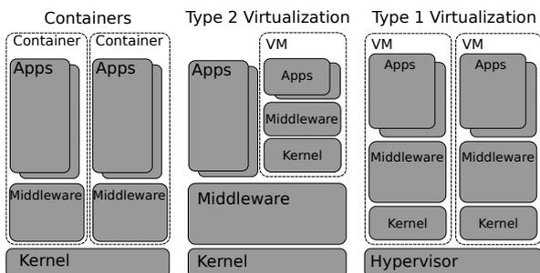
Figure 6: Android virtualization architectures. From left to right: Containers, Type 2 and Type 1 virtualization.
